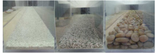
Figure 2. Details of the rough beds used for runs of type R: R1 (left), R2 (center) and R3 (right). View of the channel bed from the downstream section, i.e., right end wall in Fig. 1.
