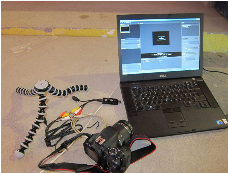
Figure 2 - Laptop computer (Windows XP, 4 GB RAM) used to receive conveyed video signal from A/D Converter DAQ board. Also shown are the Canon camera and zoom lens, the Gorillapod, cables (with USB-composite video adapter) and the “USB Conceptronic A/D Converter DAQ board”.
