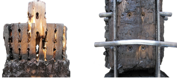
Figure 9: Failure modes of connections D01.1.R-1 (left) and D04.1.R-1 (right) in the fire tests.
