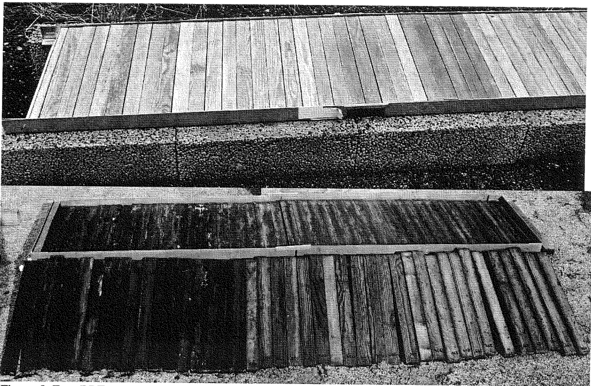
Figure 5. Top: BRE test deck in the UK and bottom: Opened up Wolman test deck in Sinzheim, Germany.
