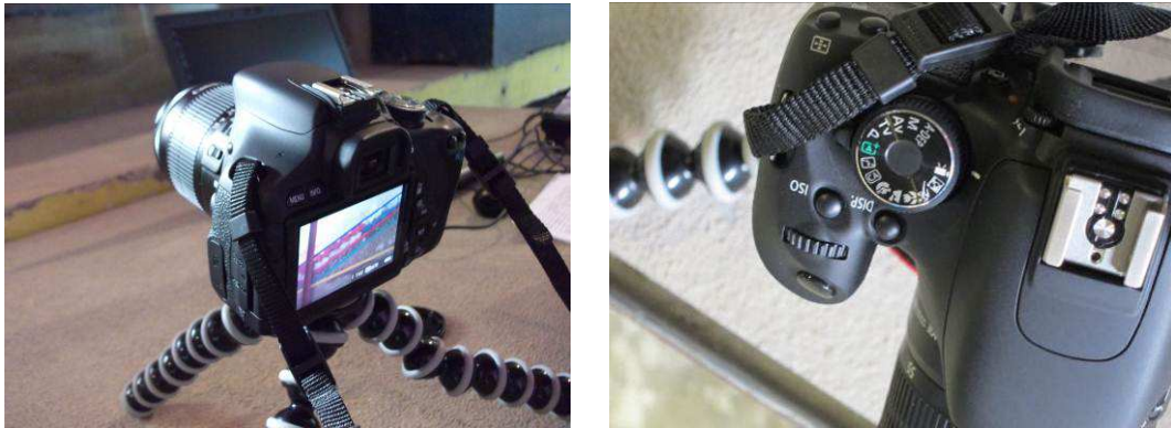
Figure 8 – Setup of camera in the final position and video mode operation selection.
