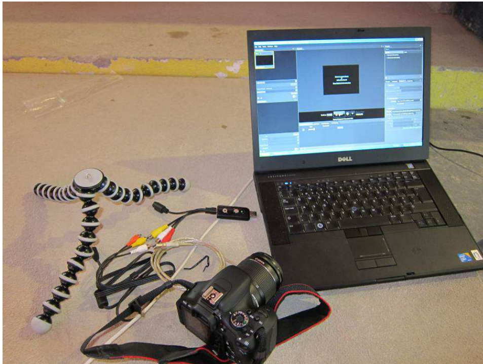
Figure 4 - Laptop computer (Windows XP, 4 GB RAM) used to receive conveyed video signal from A/D Convertor DAQ board. Also shown are the Canon camera, the Gorillapod, cables (with USB-composite video adapter) and the “USB Conceptronic A/D Convertor DAQ board”.
