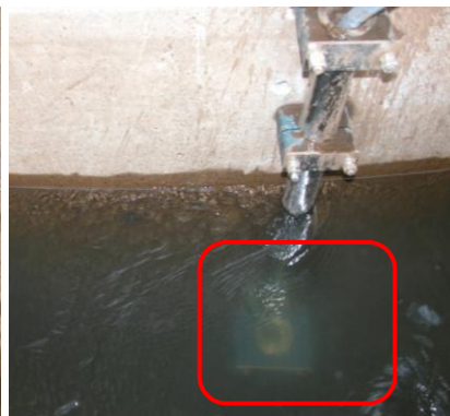
Fig. 7 – The acoustic scour meter mounted in pier P8
