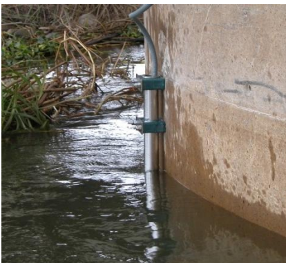
Fig. 7 – The acoustic scour meter mounted in pier P8
