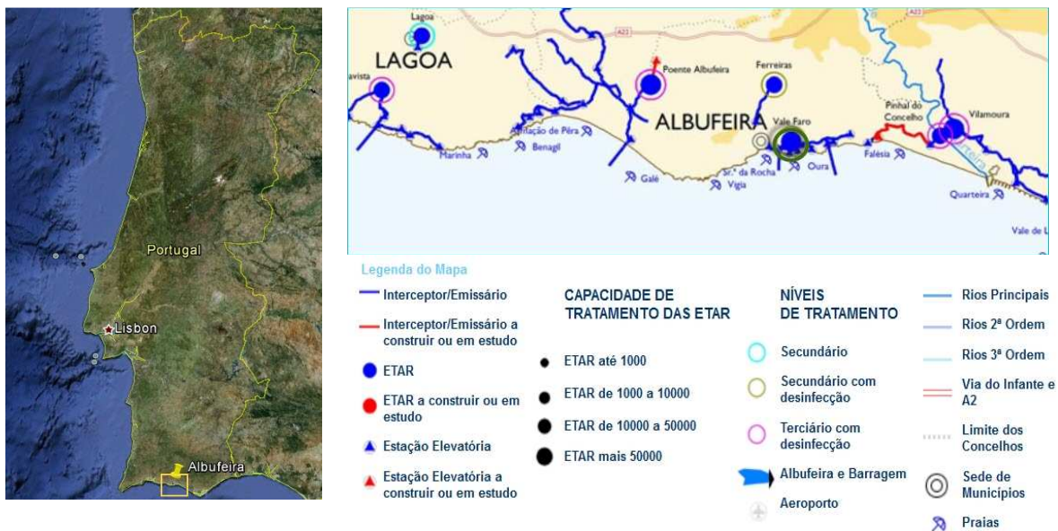
Figure 5. a) Case study location (Albufeira), b) Example of the wastewater treatment system in Algarve region (source: www.aguasdoalgarve.pt )
