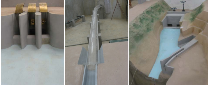
Figure 6 – Main spillway (intake and curved tunnel), auxiliary spillway and power station restitution
