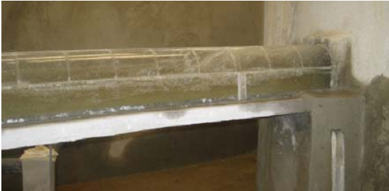
Figure 7 – Upstream part of tunnel with a strong winding flow
