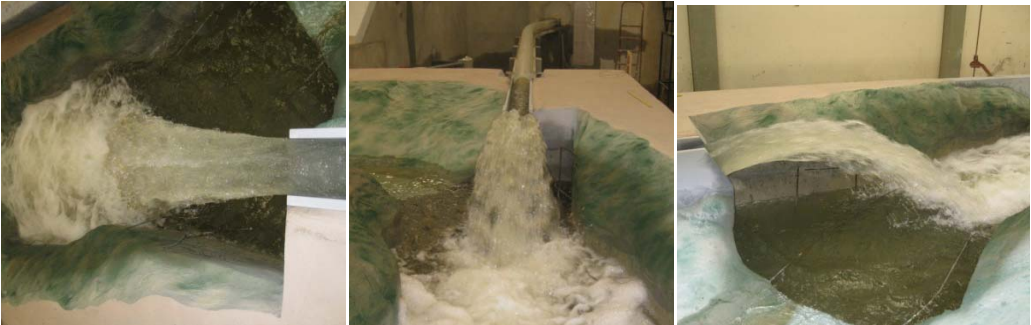
Figure 8 – Jet behaviour in the main spillway
