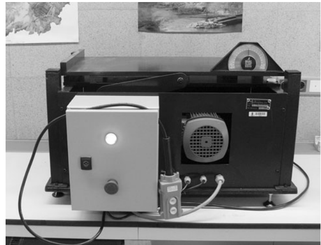
Fig. 4 Purpose built tilt testing machine for jointed rock samples, with a motorized platform that tilts at 0.4^\circ/\text{s}
