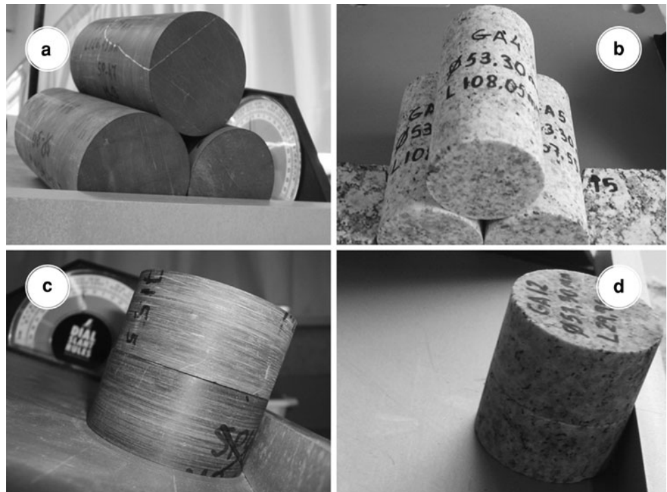
Fig. 1 Tilt tests performed on slate and granite samples
