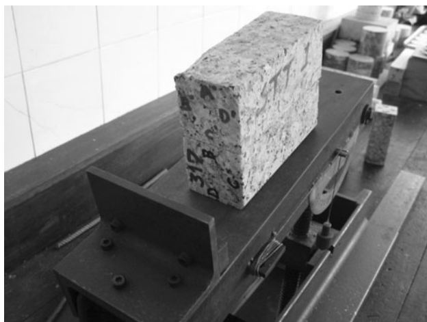
Fig. 10 Preparation for tilt test 317B–316C'
