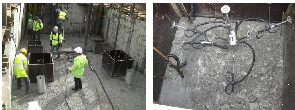
Figure 11 – General view with the strain group relative location (left), and detail five strain transducers group arrangement (right).
