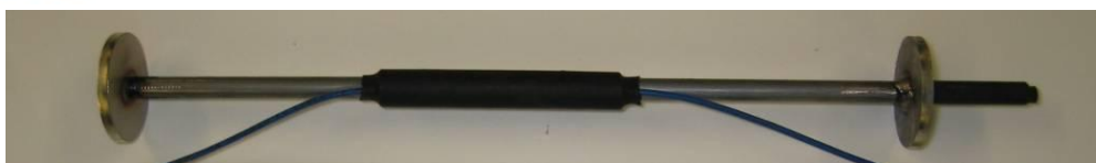
Figure 5 – Schematic representation of the optical based strain transducer to be embedded into concrete.
