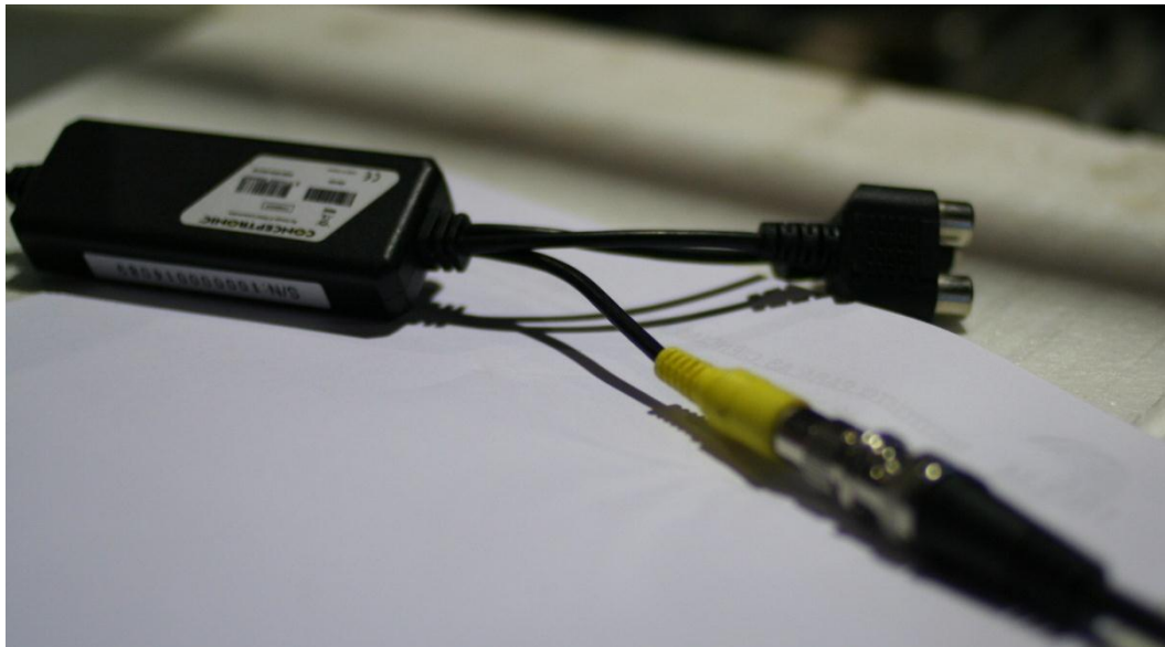
Figure 3 - COI1 flume. Cable connection (with BNC-composite video adapter) between CATV Camera and “Conceptronics A/D Converter DAQ board”.
