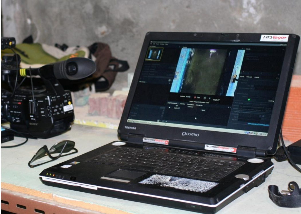
Figure 4 - COI1 flume. Laptop computer (Windows XP, 4 GB RAM) used to both receive conveyed video signal from A/D Converter DAQ board (through USB interface, decode video and send decoded signals to computer server.
