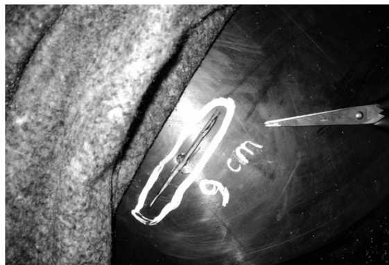
Figure 8. Shape and dimension of the tear.
