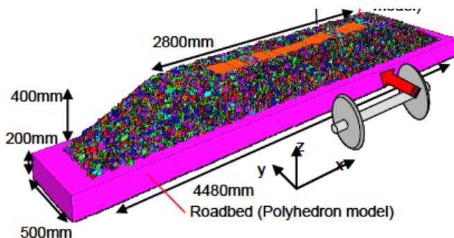
Figure 11. 3DEC model of ballasted railway track (Aikawa 2011).
