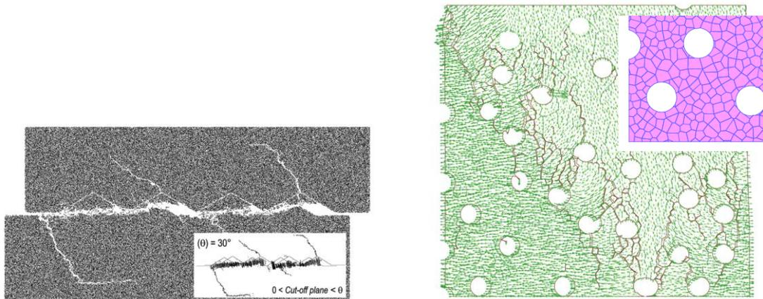
Figure 2. (left) Particle model of shear test of synthetic rock fracture profile (Asadi & Rasouli 2011); (right) UDEC model of uniaxial compression test on lithophysal tuff specimen (Damjanac et al. 2007).
