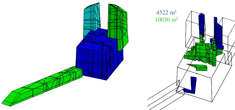
Figure 9. 3DEC model of Tindaya mountain project: (left) Excavation shapes; (right) Volumes of unstable rock in the unsupported case (Senís & Varona 2008).
