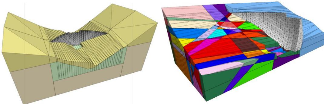
Figure 7. 3DEC model of Baixo Sabor dam: (left) global model geometry before discontinuities are inserted; (right) detail of half of the block model with rock discontinuities (Lemos & Antunes 2011).
