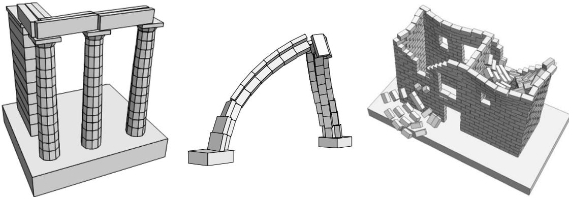
Figure 10. Rigid block models for seismic analysis of stone masonry. (left) Parthenon Pronaos (Psycharis et al. 2003); (center) free-standing arch (Lemos 2007); (right) traditional house (Alexandris et al. 2004).
