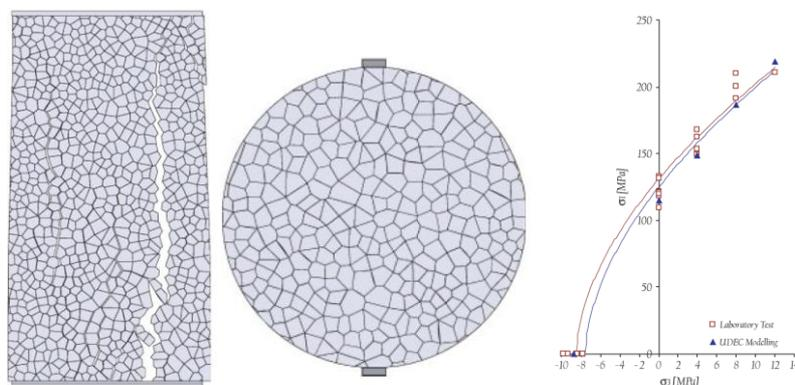
Figure 3. Rock specimens based on Voronoi polygons for simulation of uniaxial compression and Brazilian tensile tests and comparisons with experimental results (Kazerani & Zhao 2010).
