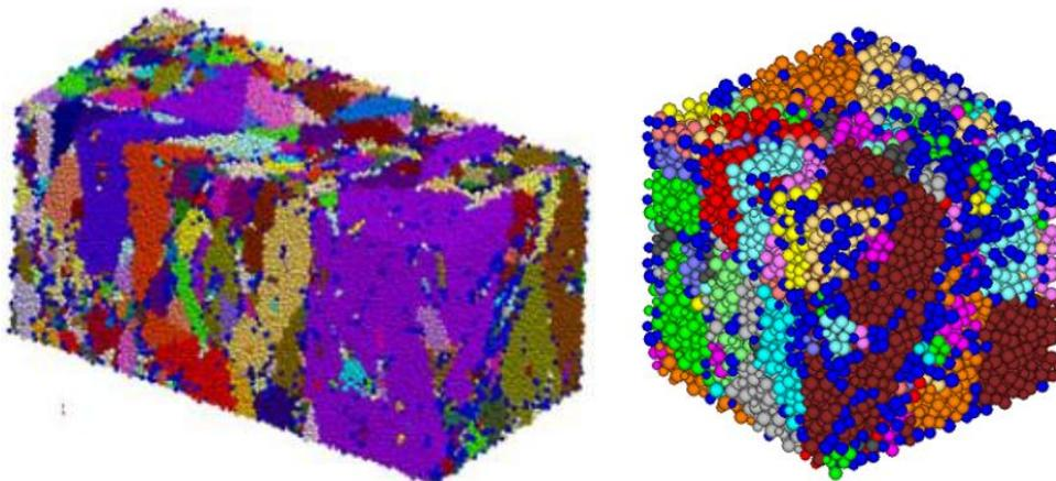
Figure 5. Three-dimensional SRM models: (left) view of the 80x40x40 m model; (right) detail view of DFN inserted on PFC brick (Mas Ivars et al. 2008).
