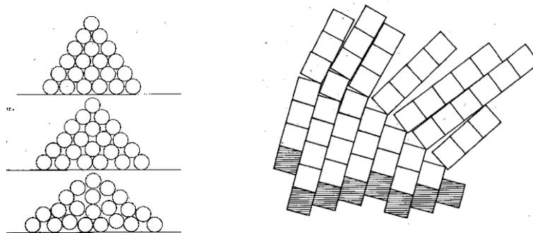
Figure 1. Two examples from Cundall's 1971 paper on the distinct element method: pile of disks and toppling failure mode of rock slope.
