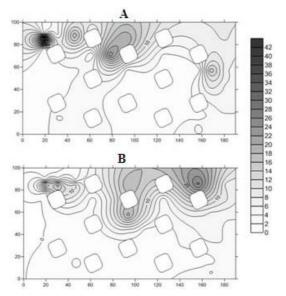
Figure 2. Contours of the vertical component of Reynolds shear stress ( $RSS_{xz}$ ) on the plane at boulders mid-height for regime 1 (A) and regime 2 (B). Values are in N.m<sup>-2</sup>. The squares represent the boulders with their position and alignment.
