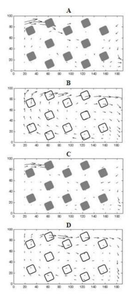
**Figure 1.** Plane velocity field in the pool: (A) regime 1 at boulders mid-height; (B), regime 1 at 21 cm from the flume bottom; (C) regime 2 at boulders mid-height; (D) regime 2 at 21 cm from the flume bottom. The squares represent the boulders with their position and alignment.
