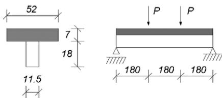
Fig. 12. Test setup of the long-term tests (dimensions in cm).
