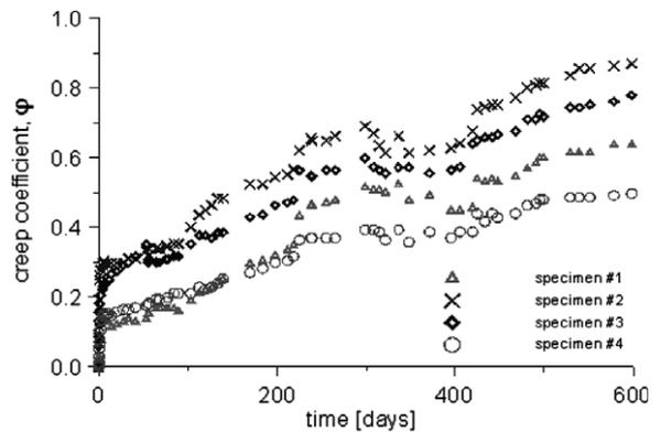
Fig. 9. Creep coefficient measured for Series I.
