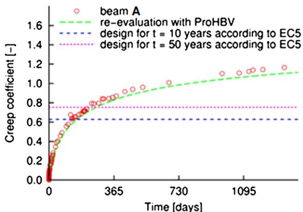
Fig. 13. Test results compared with numerical evaluations (Beam A).
