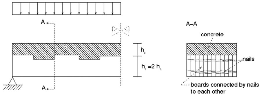
Fig. 2. Floor and cross section of the case study.
