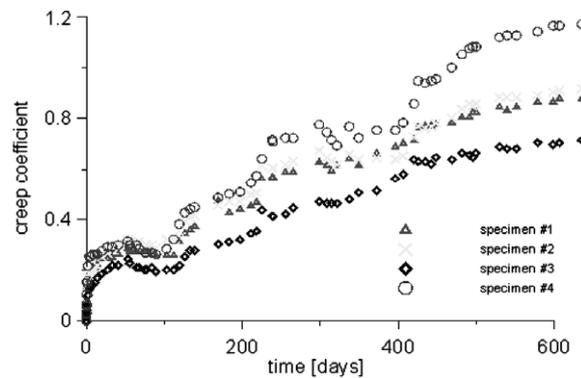
Fig. 10. Creep coefficient measured for Series H.
