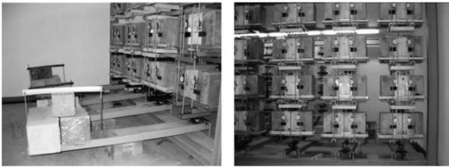
Fig. 6. Long-term tests in connection specimens.
