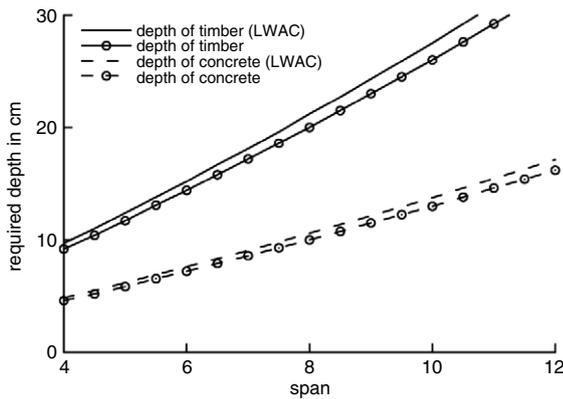
Fig. 3. Required depth of the composite members.
