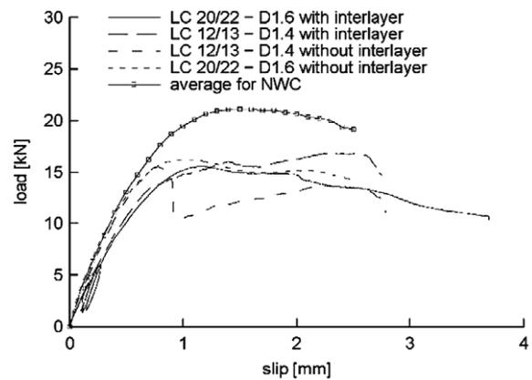
Fig. 5. Load-slip behaviour of SFS-screws in timber–concrete composite LWAC.
