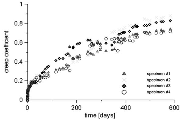
Fig. 8. Creep coefficient measured for Series Q.
