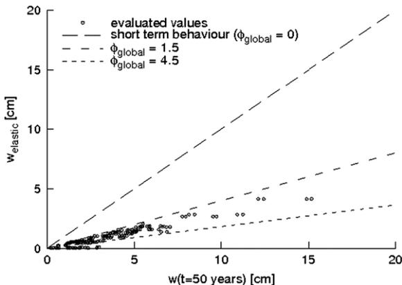
**Fig. 1.** Range of the effective creep coefficients.
