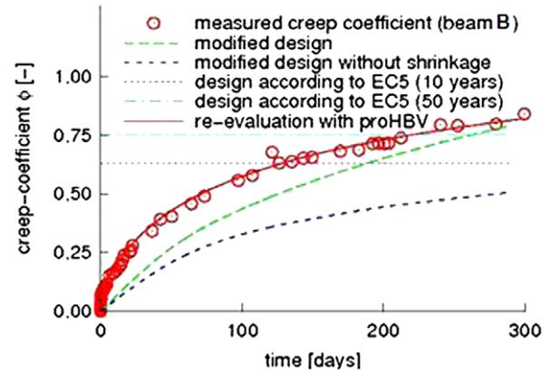
Fig. 14. Test results compared with design method according to [1,25] (Beam B).
