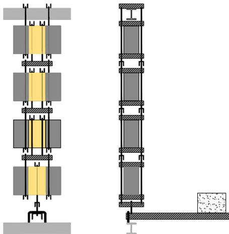
Fig. 7. Long-term shear test setup.
