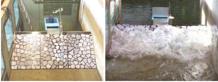
Figure 4: Equipment used and overview of wave overtopping.
