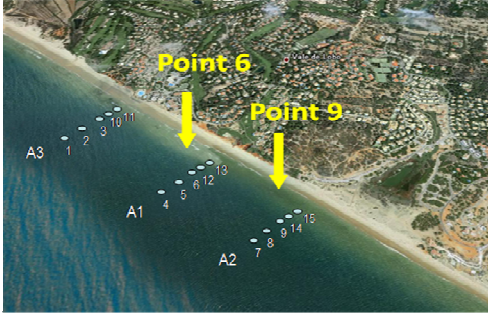
Figure 2 - Location of the 16 points in the three different cross-sections perpendicular to the beach.
