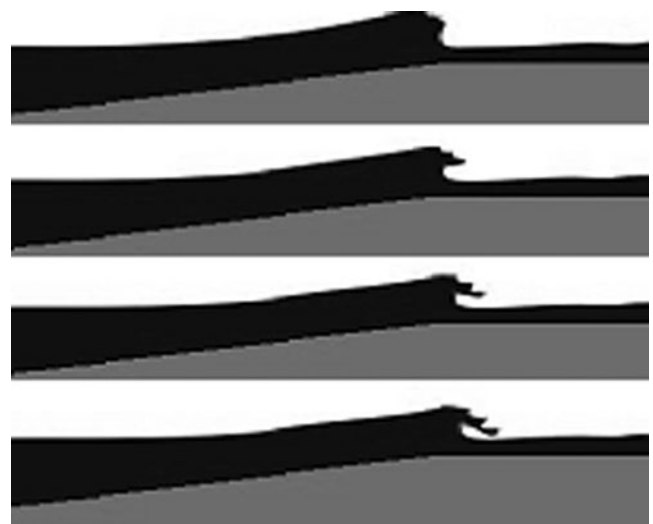
Fig. 8 Wave shape on the reef 3.20 m high ( h_{\text{init}}=7.50 m, S=1.50 m, H=1.50 m, T=9.0 s)
