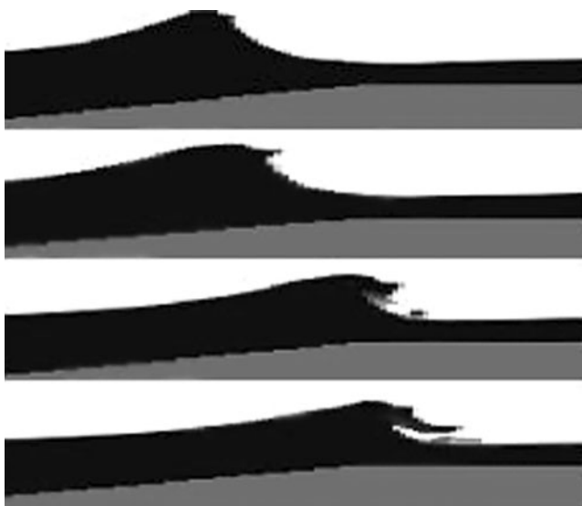
Fig. 6 Wave shape on the reef 1.90 m high ( h_{\text{init}}=7.50 m, S=1.50 m, H=1.50 m, T=9.0 s)
