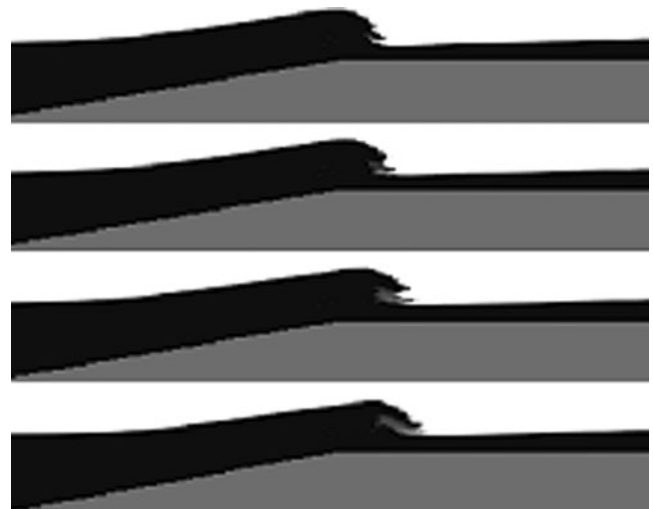
Fig. 12 Wave shape on the reef with a slope of 1:06 ( h_{init}=7.50 m, h_{reef}=3.20 m, S=1.50 m; H=1.50 m, T=9.0 s)
