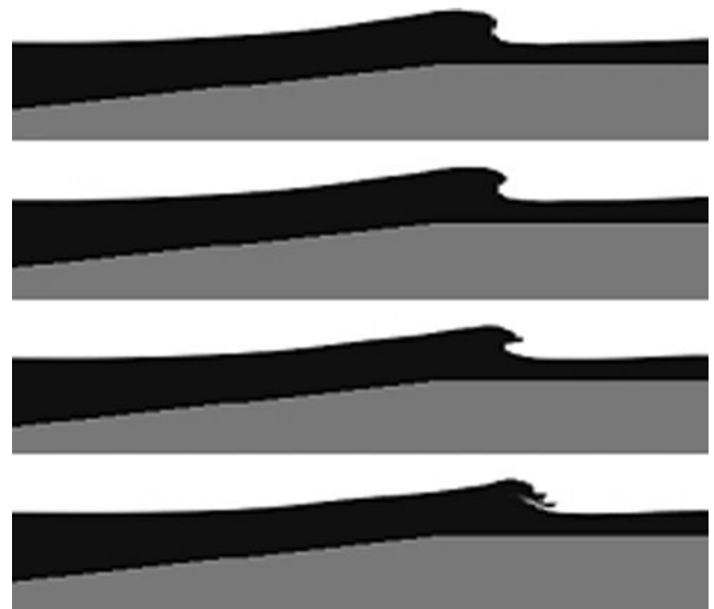
Fig. 22 Wave shape on the reef with a submergence of 2.0 m ( h_{\text{init}}=8.00 m, h_{\text{reef}}=3.20 m, H=1.50 m, T=9.0 s)
