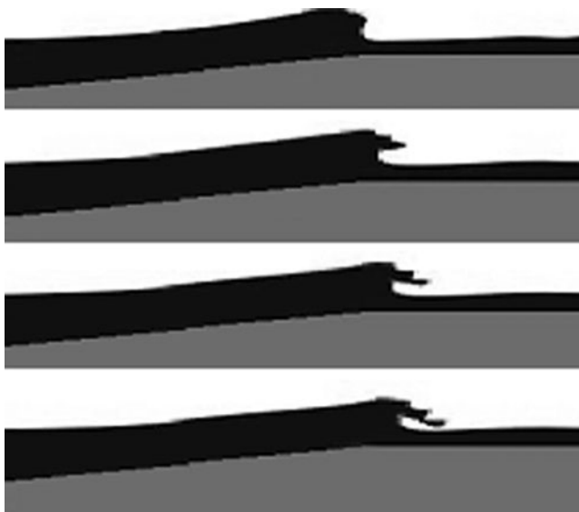
Fig. 13 Wave shape on the reef with a slope of 1:10 ( h_{init}=7.50 m, h_{reef}=3.20 m, S=1.50 m; H=1.50 m, T=9.0 s)
