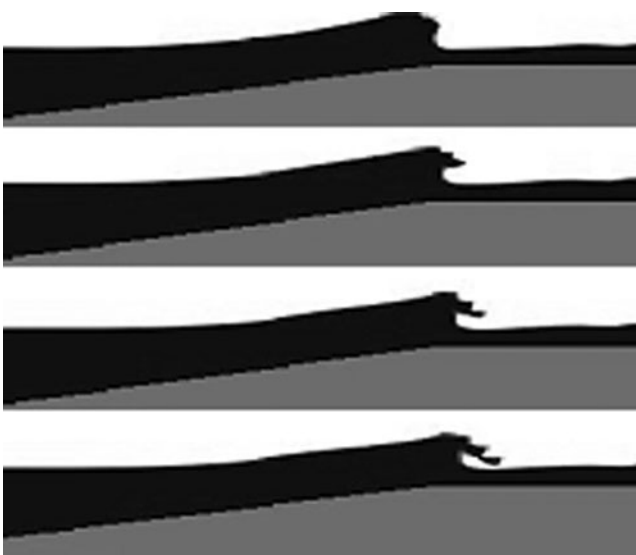
Fig. 21 Wave shape on the reef with a submergence of 1.50 m ( h_{\text{init}}=7.50 m, h_{\text{reef}}=3.20 m, H=1.50 m, T=9.0 s)
