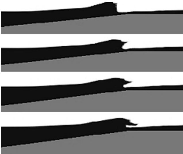
Fig. 20 Wave shape on the reef with a submergence of 1.20 m ( h_{\text{init}}=7.20 m, h_{\text{reef}}=3.20 m, H=1.50 m, T=9.0 s)
