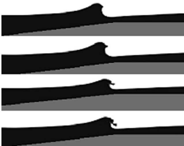
Fig. 14 Wave shape on the reef with a slope of 1:14 ( h_{init}=7.50 m, h_{reef}=3.20 m, S=1.50 m; H=1.50 m, T=9.0 s)
