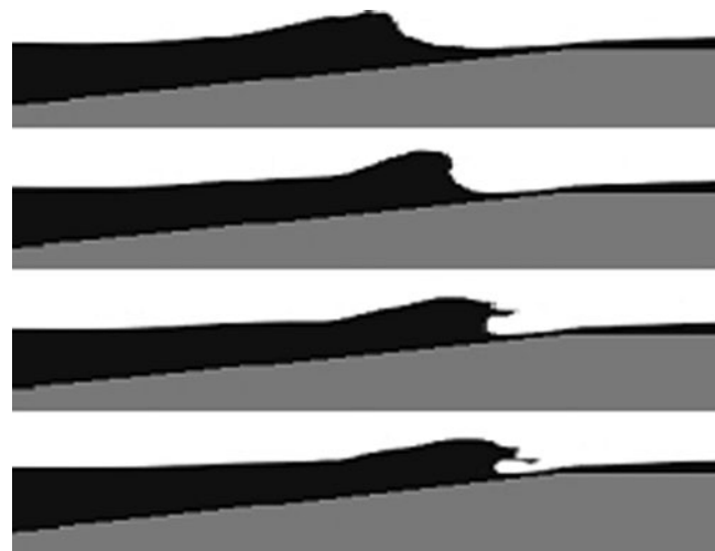
Fig. 19 Wave shape on the reef with a submergence of 0.80 m ( h_{init}=6.80 m, h_{reef}=3.20 m, H=1.50 m, T=9.0 s)
