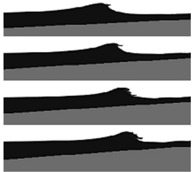
Fig. 15 Wave shape on the reef with a slope of 1:18 ( h_{init}=7.50 m, h_{reef}=3.20 m, S=1.50 m; H=1.50 m, T=9.0 s)
