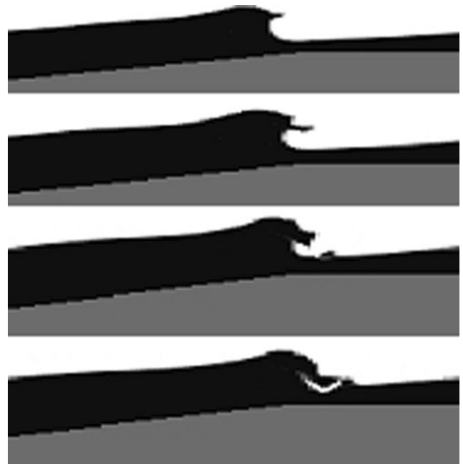
Fig. 7 Wave shape on the reef 3.90 m high ( h_{\text{init}}=7.50 m, S=1.50 m, H=1.50 m, T=9.0 s)
