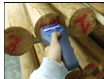
Figura 10 – Timber Grader - MTG
