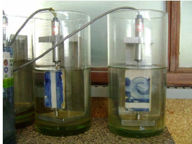
Figure 2 - Moisture expansibility measurement set-up.
