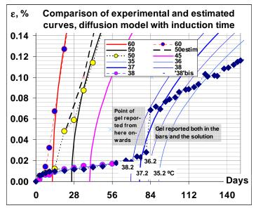
The model was tentatively applied to a case reported in literature, of a railway sleeper kept in a covered area, which displays early symptoms of ASR after 11 years. Correction for alkalinity of the cement used, temperature and humidity from meteorological data were applied, using equations referred to in the literature.
