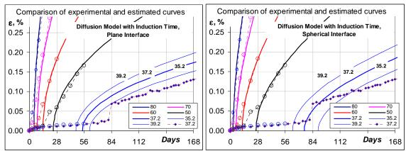
The effects of the factors temperature, alkalinity and humidity assumed models referred to in literature, or obtained by regression both of kinetic parameters for each isothermal curve and their temperature coefficients of Arrhenius plots. The correlations obtained allow estimating the strain after the induction period, for any value of the mentioned factors, under
