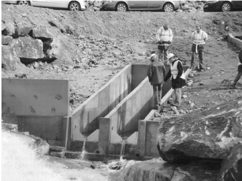
Figure 12: Flow meters near the toe of the dam. The left one measures the seepage and the right one the flow from the natural springs
