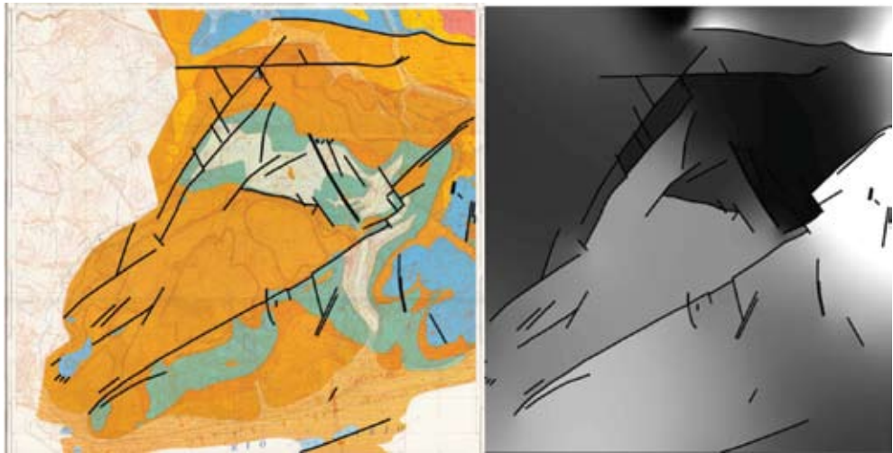
Figure 5. Faults system and interpolation of surfaces affected by it (Sheet number 3 of the Geological Map of Lisbon 1: 10000).
