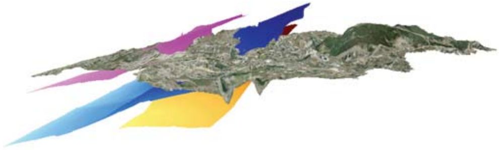
Figure 4. Example of stratigraphic layers interpolated from the correspondent point data by kriging method (Vertical exaggeration 6x).
