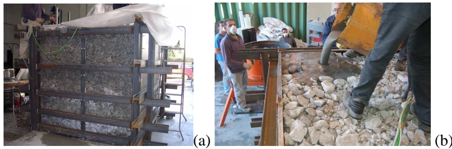
Figure 5 – Prototype before filling (a) and location of the mortar pouring (b)
