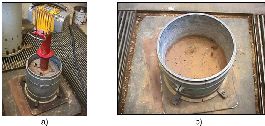
Figure 11 – a) Electric vibrating hammer and mould; b) cylindrical mould
