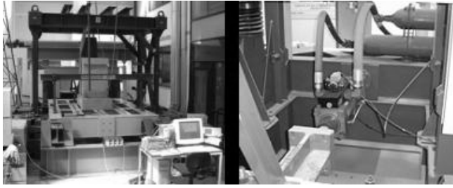
Figure 1. Overview of the shaking platform and its unidirectional hydraulic actuator.
