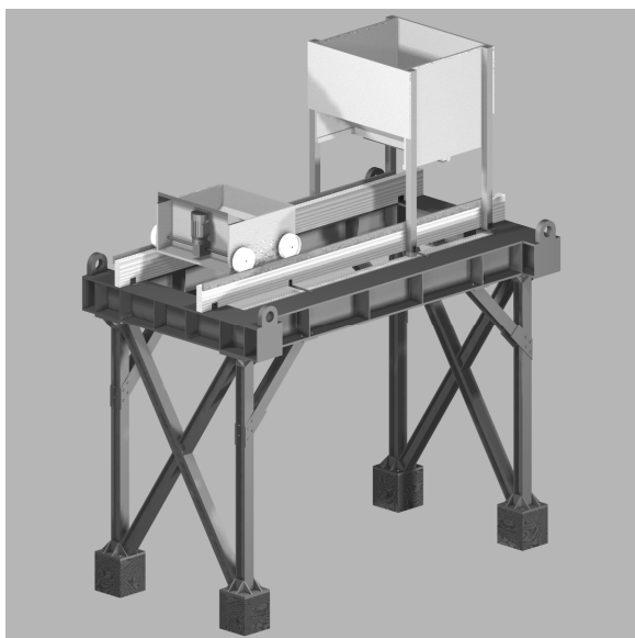
Figure 6. Schematic view of the pluviator equipment setup.
