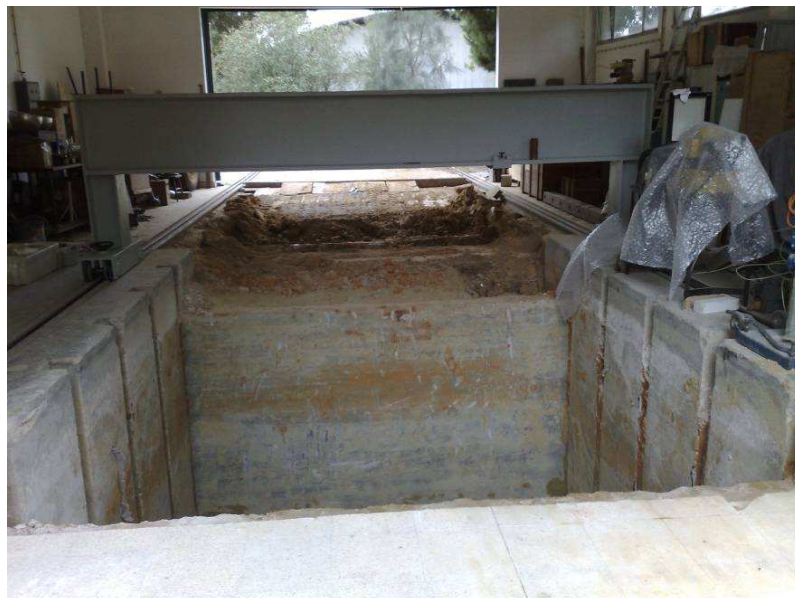
Figure 2 - Overview of the tests pit and reaction beam
