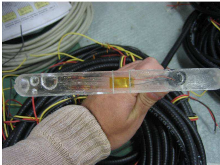
Figure 12 - Top view of the displacement transducer
