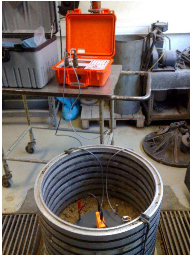
Figure 23 – Tests performed with the EDG on the Chamber DU 50
