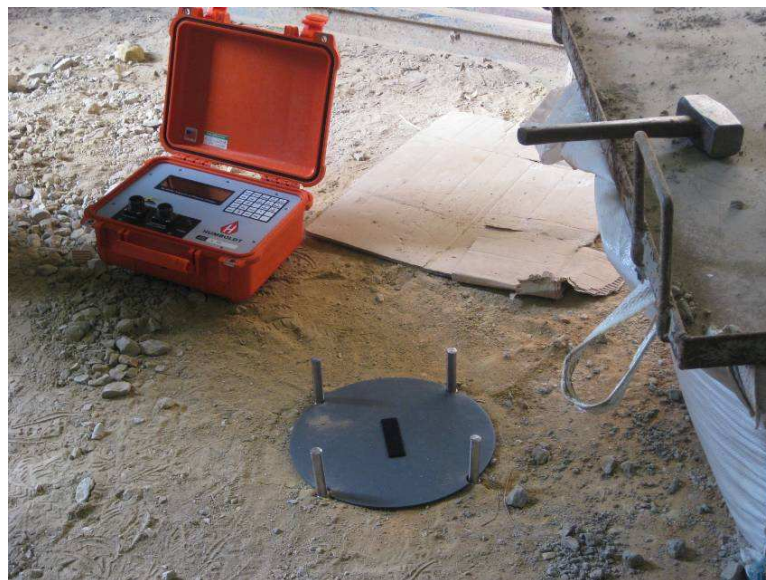
Figure 24 – EDG tests performed at LNEC tests pit
