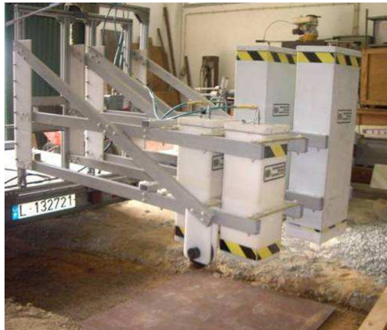
Figure 21 - GPR measurement – metal plate calibration
