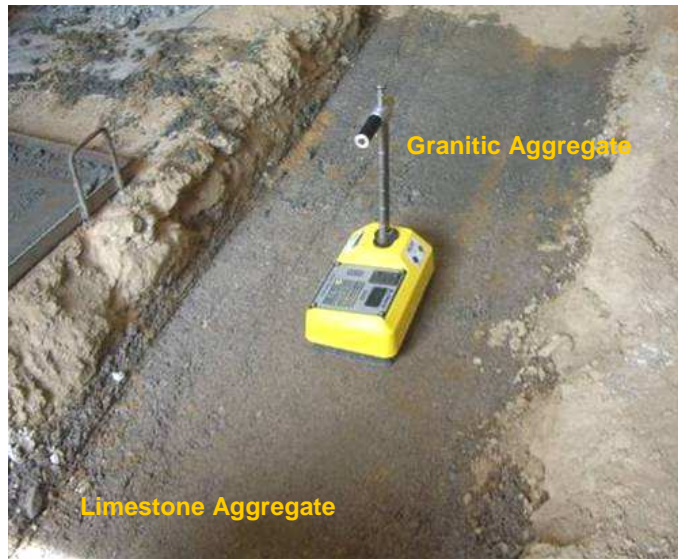
Figure 20 - Experimental site - Troxler measurements
