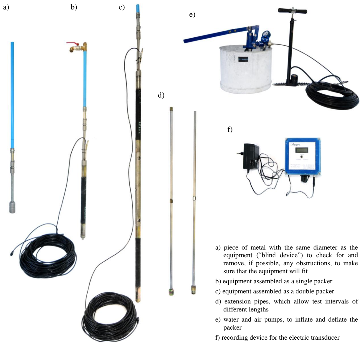
Figure 4.3 – Main parts of the equipment.
