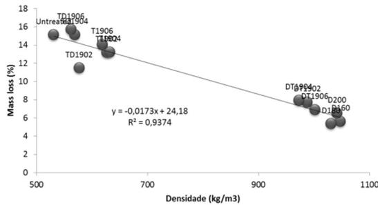
Fig. 6: Relation between mass loss due to termite attack and wood density.
