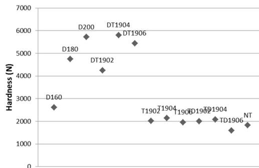
Fig. 2: MOE, Bending strength and Janka hardness changes in relation to untreated wood for: densified (D), heat treated (T), heat treated after densification (DT) and heat treated.
