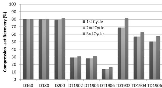
Fig. 1: Compression-set recovery after three wetting cycles for wood: densified (D), heat treated after densification (DT) and heat treated before densification (TD).
