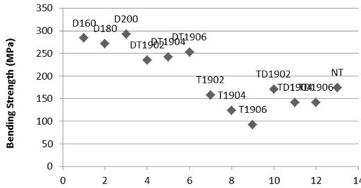
Fig. 3: Bending Strength for wood: untreated (NT), densified (D), heat treated (T), heat treated after densification (DT) and heat treated before densification (TD).
