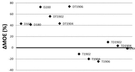
Fig. 4: MOE changes in relation to untreated wood for: densified (D), heat treated (T), heat treated after densification (DT) and heat treated before densification (TD).
