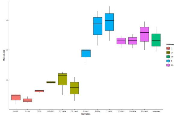
Fig. 5: Mass loss (%) due to termite attack on wood: untreated, densified (D), heat treated (T), heat treated after densification (DT) and heat treated before densification (TD).
