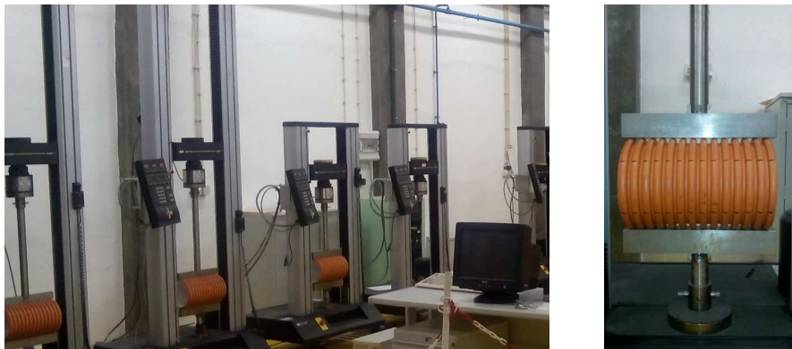
Fig. 1 – Typical experimental assembly for creep tests: a) overview; b) detail of a specimen under test
