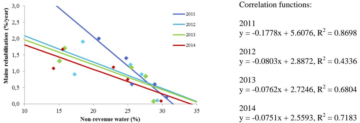
**Figure 7.** Linear regression between NRW and mains rehabilitation in AGS' utilities (2011-2014).
