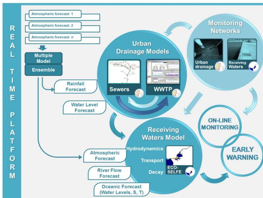
**Figure 1.** Conceptual scheme of the real-time monitoring and forecasting system.
