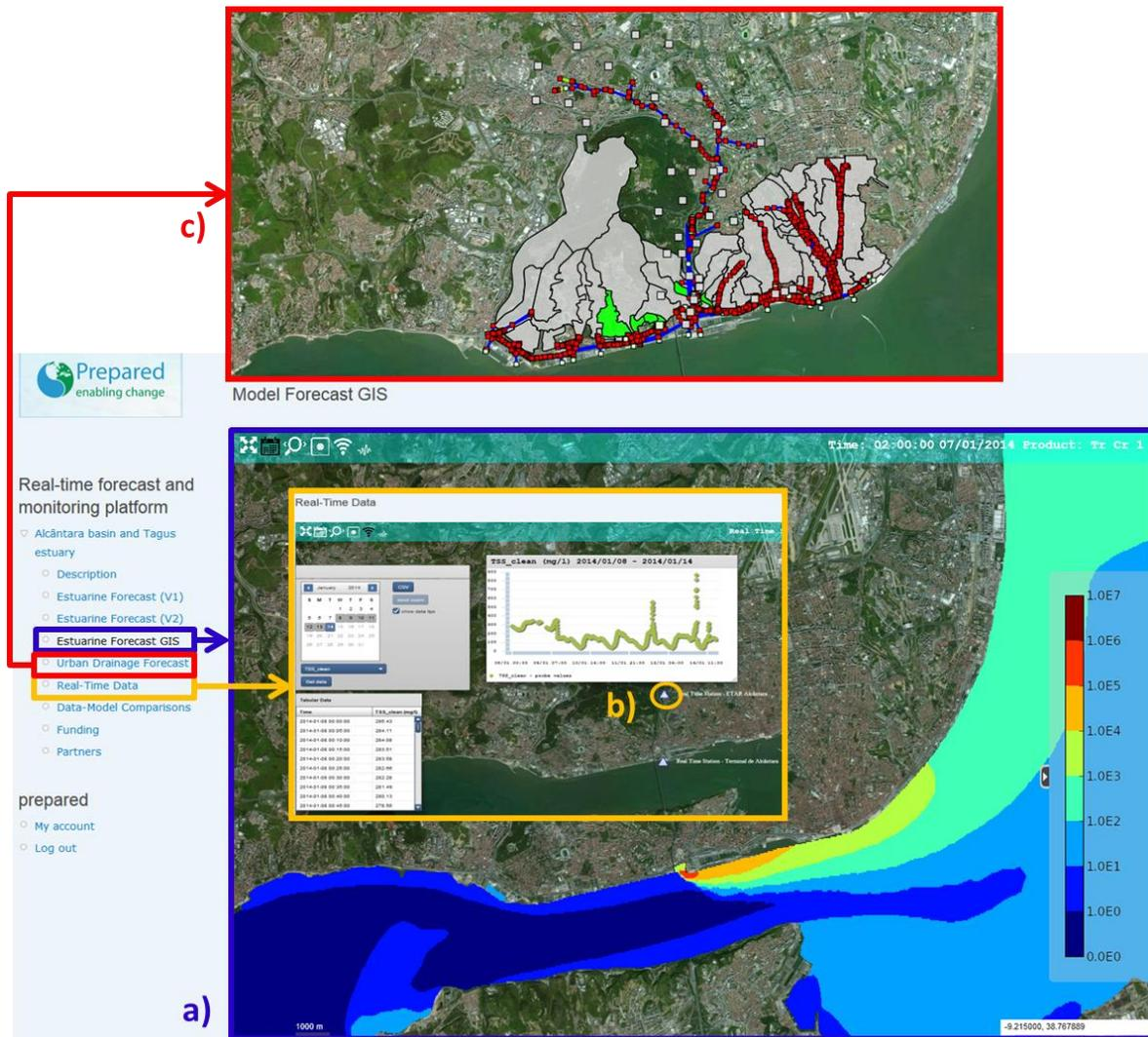
**Figure 3.** WIFF interface showing: a) faecal concentration forecasts in the estuary; b) the access to data from the on-line water quality stations and; c) the urban drainage network.
