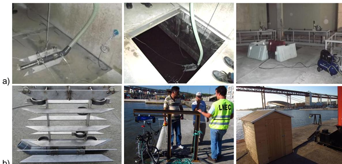
**Figure 2.** Water quality monitoring stations: a) in the sewer (WWTP inlet); b) in the estuary.
