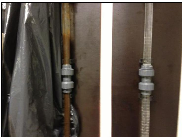
Figure 6-2 The effect of NOM removal on the biofilm formation: biofilm grown in raw water (left) and in filtered water (right)
