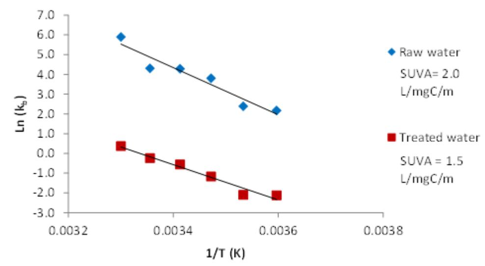
Figure 7-1 Arrhenius plot showing the influence of temperature on chlorine bulk decay coefficients
