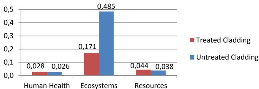
*Figure 3: Environmental impact comparison of the claddings in normalised damage category*
