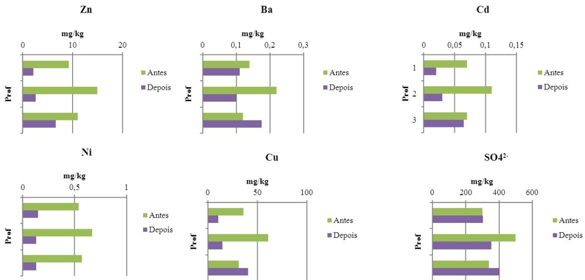
Figure 6 – Results on soil samples leachates, collected before and after nZVI injection at zone III.
