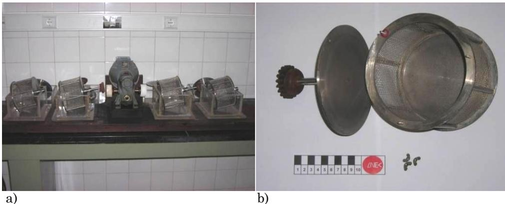
Figure 2. Equipment used for SDT tests: a) general view and b) detail of one of the stainless steel drums
