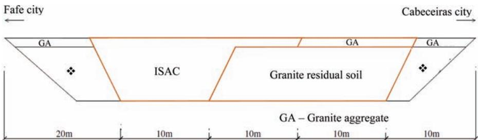
FIG. 10—Longitudinal profile of the full-scale field trial.
