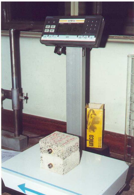
Figure 5-Measuring mass variation of Yj1 specimen (with mortar joint - block/block)
